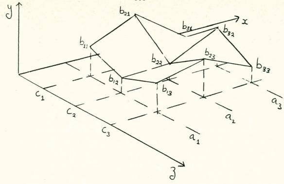
A mesh is defined on x and z with knots at  $(a_1, c_1)$  etc. Each value of (x, z) can be represented as a convex linear combination of the four adjacent knots. If we call the weight given to the knot  $(a_i, c_j)$  wij then the point  $((a_1 + a_2)/2, (c_1 + c_2)/2)$  could be represented by
