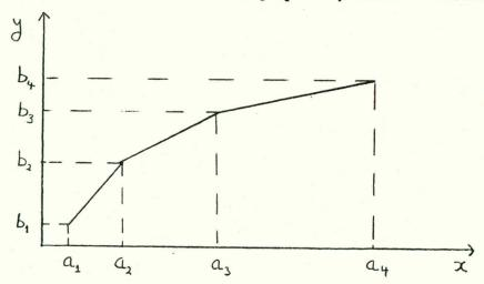
The points  $a_1$ ,  $a_2$ ,  $a_3$ ,  $a_4$  on the x-axis where the line is broken are called knots. Any given value of x can be represented as a convex linear combination of the knot values:
